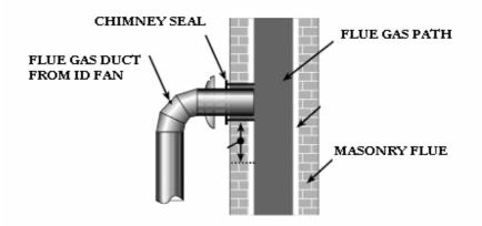
Generally the opening on the chimney flue would be larger compared to the duct size to accommodate the radial expansion of the duct due to thermal expansion and also the possible misalignments. However if this gap is not properly sealed, it could lead to the escape of flue gas along with ash particles. In one of the boiler installations, due to the ash leakage from these gaps the maintenance lift could not be operated.
