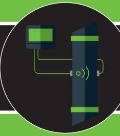
Acospector sends and receives acoustic signals which are then analysed in a server environment.
