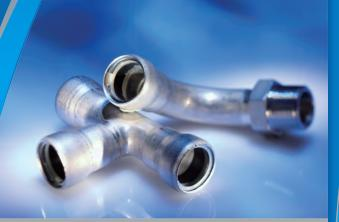
Profile ► Stainless Steel Press Fittings Materials ► SUS304 Stainless Steel Certificates ► JSSA- SAS 322, JWWA Pressure rating ► 150 PSI (10 kg/cm<sup>2</sup>)
