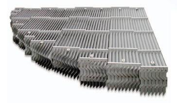
Complex Vane Pack designs provide special separation channels to allow disengagement of liquid and drainage from the vane surface which increases the capacity. These profiles are therefore used when equipment size is critical, for example in de-bottlenecking of existing equipment.
