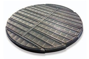
They are produced as multiple layers of knitted mesh making it a dense pack and presenting a large surface area to the droplets entrained in the gas stream. The separation of the droplets is achieved by impingement on, and capture by, the wires of the mesh where the droplets coalesce and drain.
