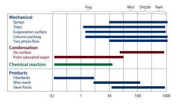
Mist elimination systems provided by Omega Separations prove to be an effective solution to liquid entrainment problems in many types of equipment including:
