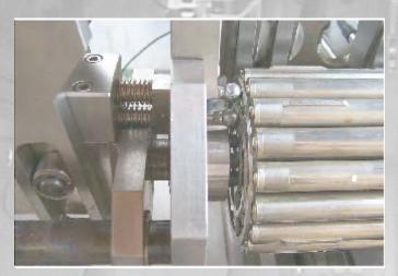
The Fuel Envelope MEasuring Rig (FEMER) was designed as a cost effective means of augmenting fuel inspection operations with the ability to measure the outer envelope of a spent fuel bundle to determine its length, element bow, bearing pad wear, and end plate deformation. In operation, the FEMER rests on the inspection table at the bottom of a fuel bay and attaches to
