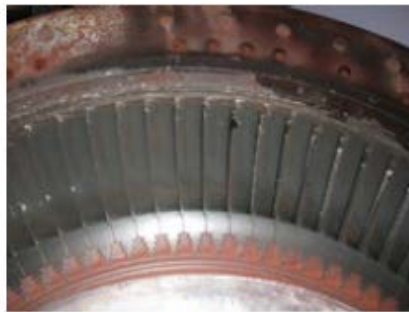
2. Collateral damage from the bucket liberation is in evidence at the trailing edges of the second-stage airfoils
