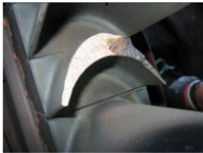
1. Two independent studies traced the root cause of the Row 2 bucket failure to stress corrosion cracking and fatigue
