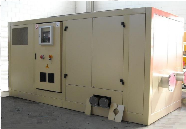
Tailor made enclosure installed on a compressor
