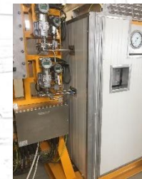
Final solution applied on the skid, noise reduction of 30 dB(A) ~
