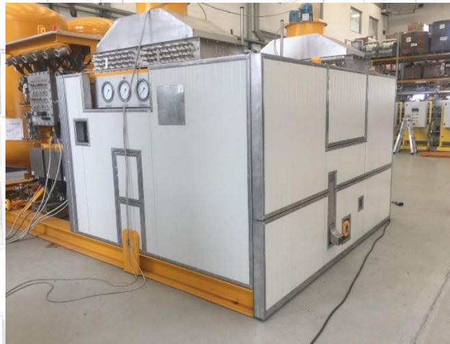
Final solution applied on the skid, noise reduction of 30 dB(A) ~
