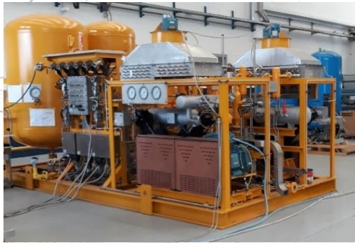
Starting screw compressor situation with noise level at 120 dB(A) ~
