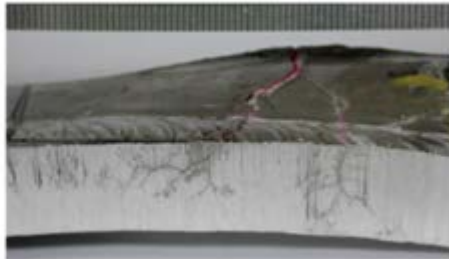
Figure 4: Subsurface branched cracking found in the vicinity of the failure.
