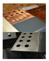
A typical bus bar has four distinct faces that require silver plating. Prior to installing the semi-automated workstation, this was done manually, one face at a time, requiring an operator to move a hand-held plating tool (anode) back and forth across the surface being plated until the desired silver thickness was
