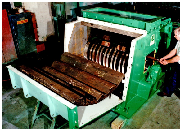
The curved breaker block assembly matches the hammer circle profile.
