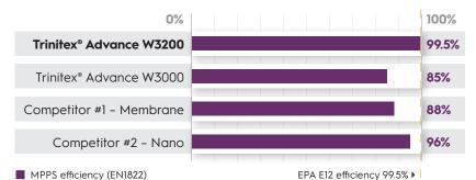
**Trinitex® Advance W3200 is a true E12** according to EN1822, reaching >99.5% MPPS efficiency.
