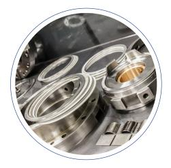
The bearings are completely dismantled; the components are cleaned & measured. In every case the naked bearings are replaced & the rest of the components such as damping springs & bearing bushes are carefully inspected for reuse, in other case they are replaced.
