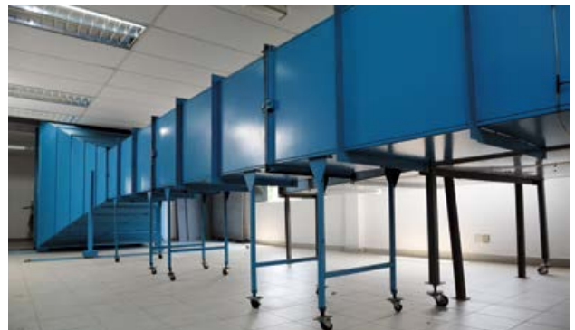
Testing (Testing Duct based on ISO 7235)
