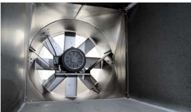
Auxiliary fan for volume measurement purpose (Test laboratory for ISO 7235)
