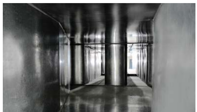
Silencer (attenuator) test assembly
