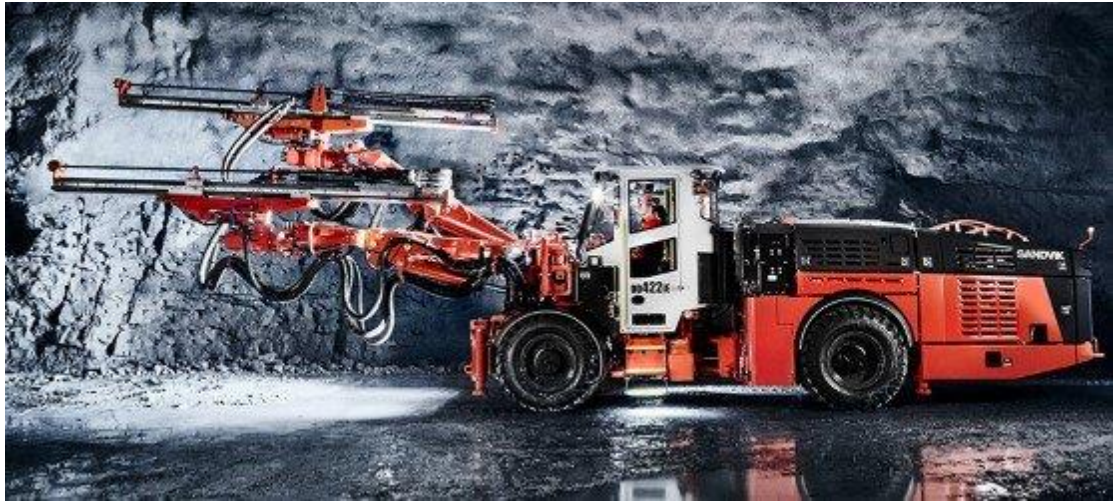
DD422E (Electric) Sandvik Jumbo Drill
