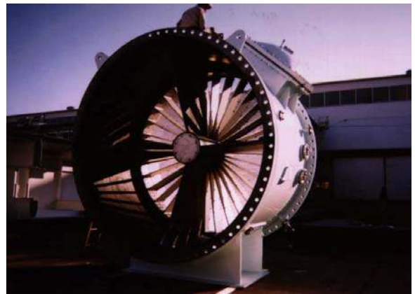
Debris Filter – Nominal Diameter 3200 mm (Japan)
