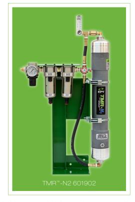
nitrogen sweeps across the reservoir, it will absorb water vapor which is forced out of lubricant as it moves towards moisture equilibrium with the Nitrogen on top of it.
